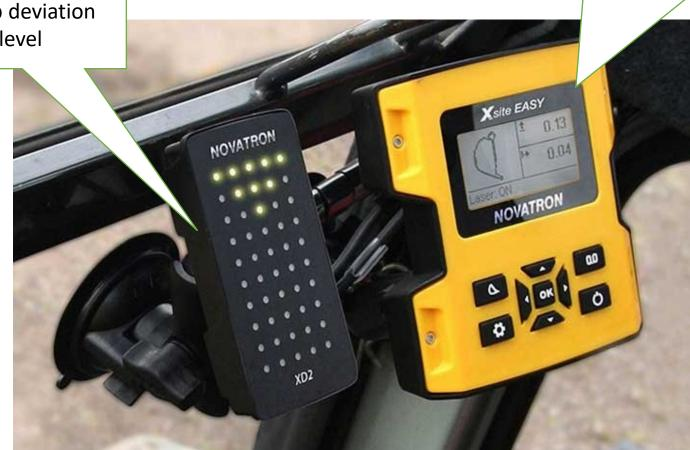
LED display indicate cutter pump deviation from target level
